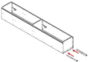
**7.** Place the door and frame assembly (Ref. No. 7) over the locker body. Make certain that body sides are inside frames.
