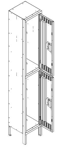
**10.** Anchor units to wall or floor. The units are not intended to stand free and may topple if not secured. Units standing back to back should be bolted back to back.
