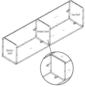
**5.** Bolt the right side (Ref. No. 6) to the back so that the side flange fits around the back also attaching to the top, middle and bottom shelves using thirteen nuts and bolts if the locker has no legs and fifteen nuts and bolts for a locker with legs. Attach the remaining hooks to the right side over the flange of the shelves using two nuts and bolts on each hook.
