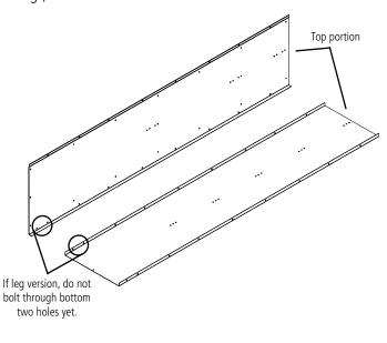
**4.** Bolt the top, middle and bottom (Ref. No. 4) to the back and side using four bolts and nuts each. Coat hooks will need to be attached over the flange of the shelves as shown. Use two bolts and nuts per each coat hook.
