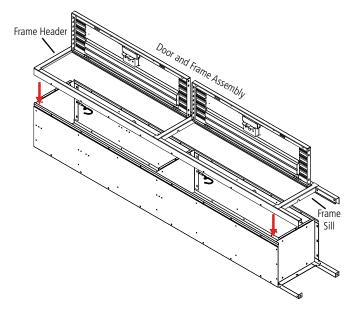
**8.** If joining units side by side, temporarily install only one bolt and nut in the frame(s) that will be joined to the adjacent locker frame(s). If locker is just a single unit, finish attaching the frame using twenty bolts and nuts. Check and tighten all permanent bolts.
